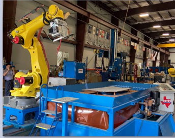
(l) Ingalls' current forming process using line heating; (c) Automated plate-shaping system developed by Navy ManTech; (r) Plate formed by Navy ManTech system in approximately 4 hours; the manual process to form the same plate takes nearly 54 hours
