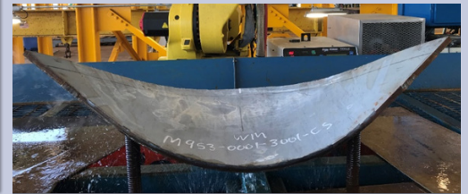
(l) Ingalls' current forming process using line heating; (c) Automated plate-shaping system developed by Navy ManTech; (r) Plate formed by Navy ManTech system in approximately 4 hours; the manual process to form the same plate takes nearly 54 hours
