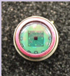
(c) Packaged Optoelectronic sensor used for sensing laser data in TALON free space optic communication system
