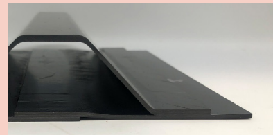
(r) Full Width Induction Welding- Overlap joint and stiffener rib joint shown
